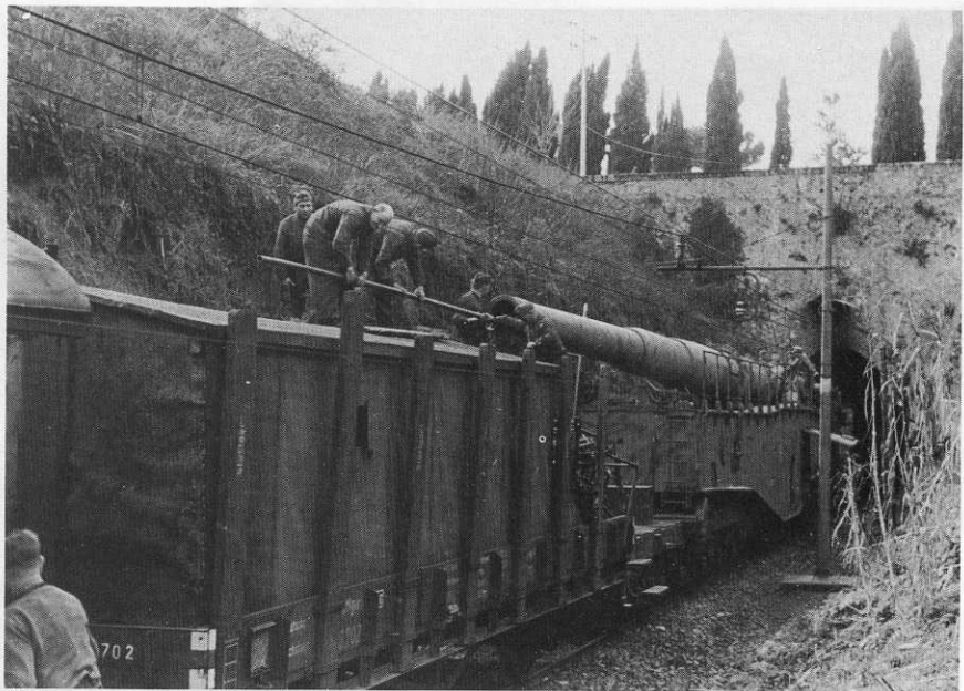
In come the big guns — the 280mm K5(E) railway Kanone weighing 218 tonnes. Its 21.54-metre barrel could launch a 255kg shell up to 36 miles. (Bundesarchiv)
